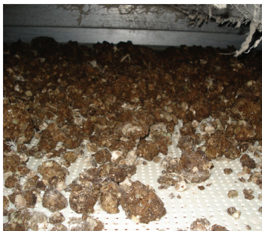
Figure 4. Perforated Cross-conveyor Belt
