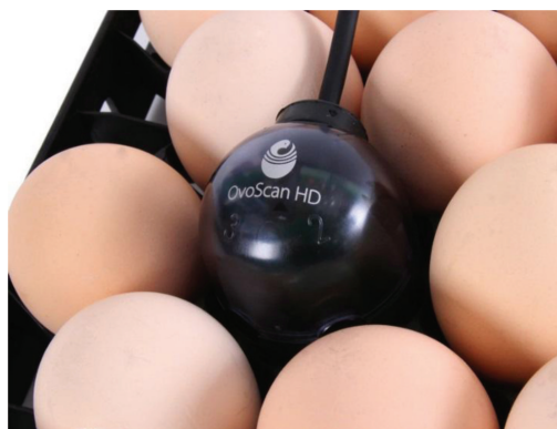
Figure 1: The system for real-time monitoring of the egg shell temperature (OvoScan™, Petersime) during incubation (Berckmans et al., 2008, Romanini et al., 2013)
